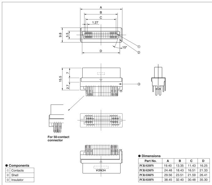
Mating connectors: PCR-E series of PCB-side right-angle DIP type connectors
