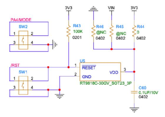
Of note in this design, the VDD pin of the RT9818C is connected to 3V3. The design is configurable by moving a zero-ohm resistor to disable supervisory reset (by connecting to GND) or to use VIN. Note that the RT9818C has a maximum input voltage of 6V which is compatible with the Photon 2. Keep this in mind if using VIN on designs that have larger VIN voltages.
