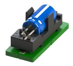
KYOCERA AVX continues to think outside the box and push the boundaries of the connector market. Our 9115 series of SMT capacitor holders allows manufacturers to eliminate hand soldering and improve production efficiency. Utilizing our proven insulation displacement (IDC) technology, we are able to safely and efficiently connect a capacitor to the PCB without the need for manual processes.
