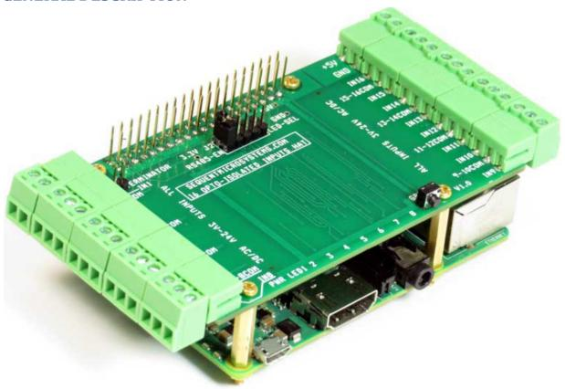
The Sixteen LV Inputs card is a stackable expansion card for Raspberry Pi. It is compatible with all Raspberry Pi versions from Zero to 5. It offers a compact and inexpensive solution for adding up to 128 universal inputs to your Raspberry Pi project. Optically isolated inputs can process AC or DC signals from 3V to 48V.
