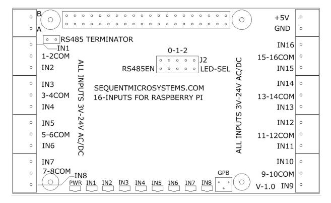
The Sixteen LV Inputs card comes with appropriate mounting hardware. Up to eight cards can be stacked on top of one Raspberry Pi.
