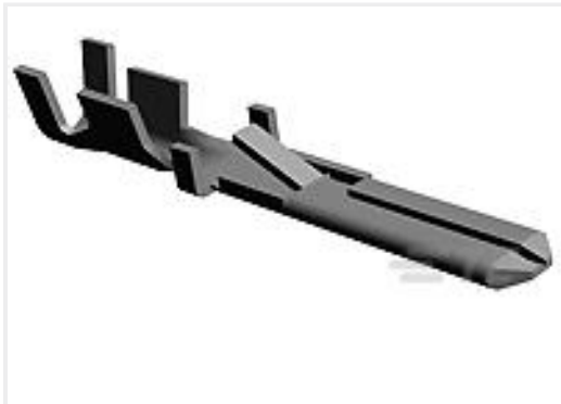
TE Part #928931-2 FF 110 (2.8 X 0.8 MM) TAB PTP CUZN30
