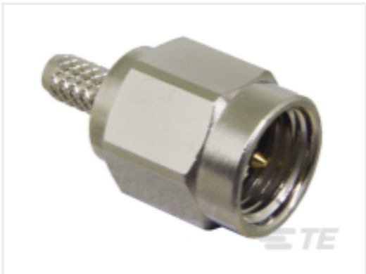
TE Part #CONSMA007 SMA Plug 50 Ohm Cable Crimp
