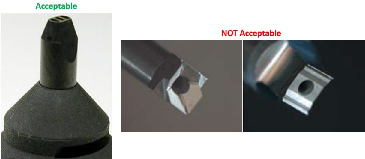
Figure 5: Acceptable vs. NOT Acceptable Tip Shapes
