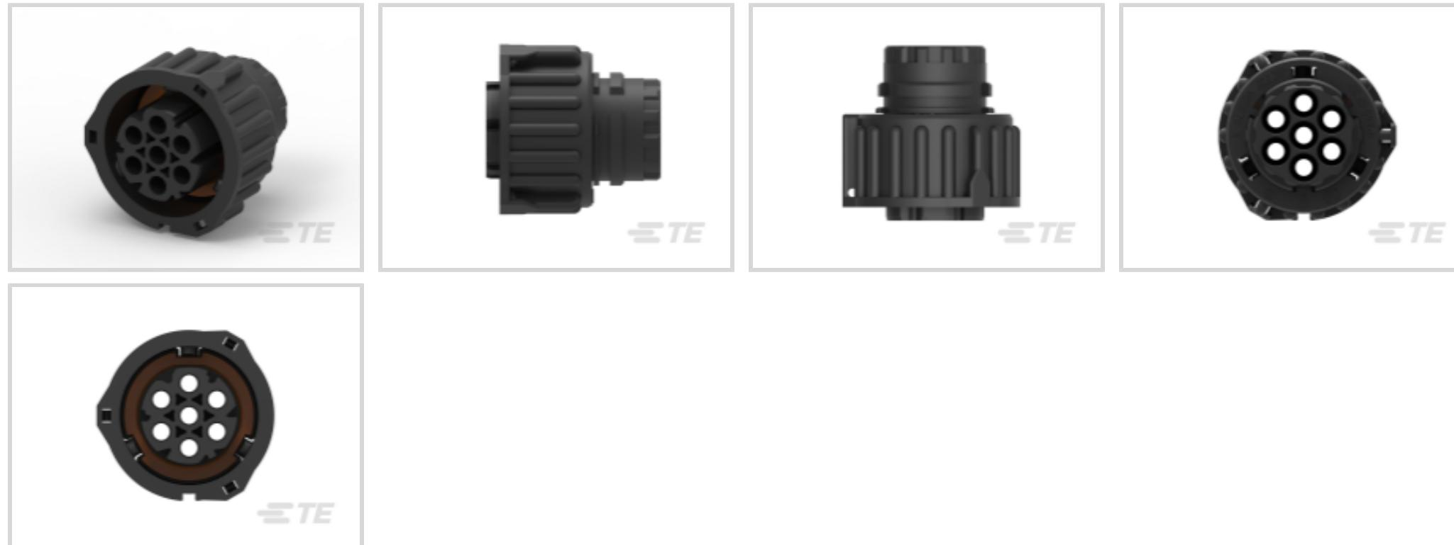
Nominal Voltage Architecture: **12 V, 24 V, 48 V**Connector & Housing Type: **Housing for Female Terminals**Number of Positions: **7**Sealable: **Yes**Operating Temperature Range: **-40 – 120 °C [ -40 – 248 °F ]**[All Circular DIN Housings \(59\)](#)
