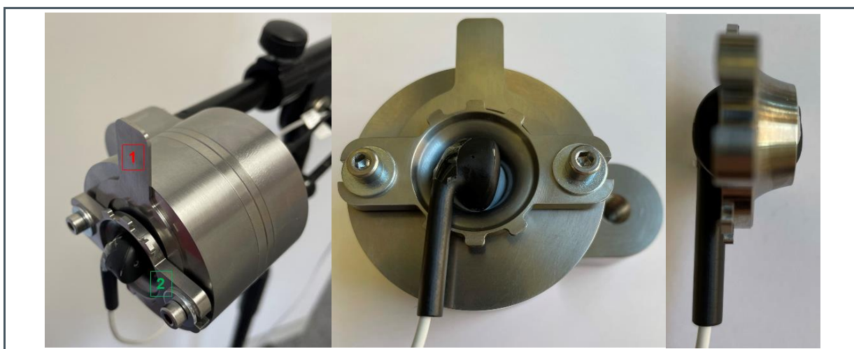
Figure 125: Leaky Measurement Adapter (LMU) Measurement
