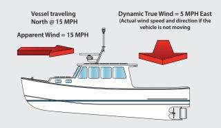
Airmar's WX Series products are the only all-in-one unit to offer dynamic true and apparent wind speeds without additional sensors.
