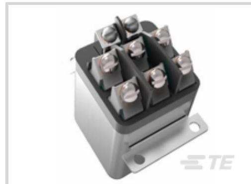
Relay & Contactor Type: **General Purpose Power Relay**Coil Magnetic System: **Non-Polarized, Monostable**Contact Arrangement: **3 Form X 3PST-NO-DM**Current Type: **AC**Contact Current Rating: **35 A**
