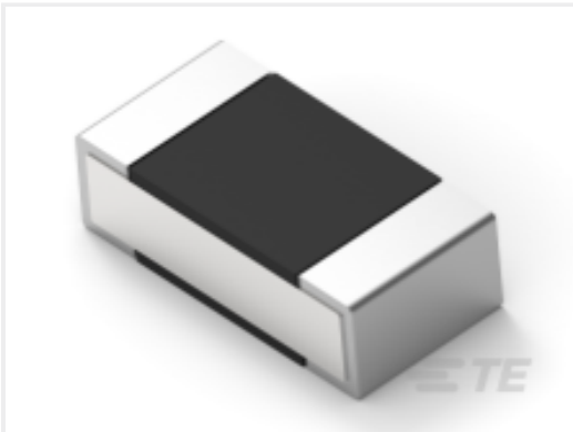
TE Part #8-2176306-4 RP 1E 0.1W 8K45 0.1% 25PPM 5K RL
