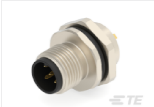
TE Part #T4132012051-000 M12,FRONT MOUNT,MALE,A,5P, SOLDER WIRE
