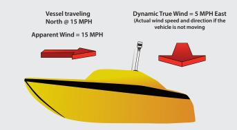
Airmar's WX Series products are the only all-in-one unit to offer dynamic true and apparent wind speeds without additional sensors.
