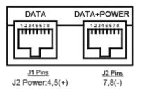
PoE injector wiring Data, Data+Power, RJ45 x 2
