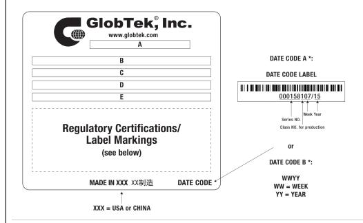
A=PoE, Passive Power Injector B=P/N: (料号) GT-96180-1824-T3-PP C=Model (型号) GT-96180-1830-6.0-T3-PP D=Input (输入)100-240V~, 50-60 Hz, 0.6A E=Output (输出)24.0 V == 0.75 A, 18.00W
