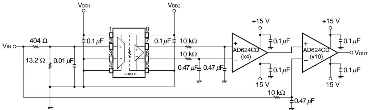
**Fig. 3 I<sub>DD1</sub> Test Circuit**
