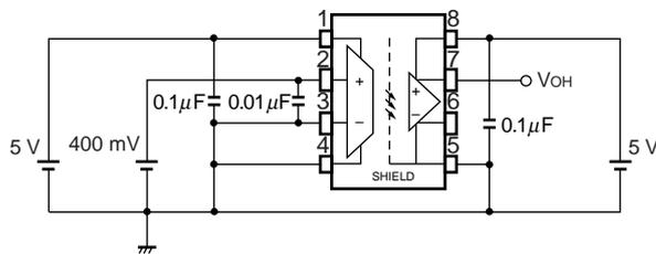
**Fig. 7 |I<sub>osc</sub>| Test Circuit**
