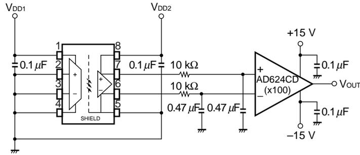
**Fig. 2 NL200, G Test Circuit**
