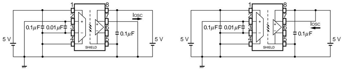
**Fig. 8 t<sub>PD</sub> Test Circuit**
