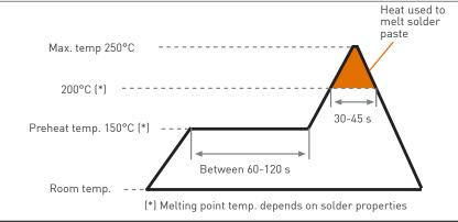
The recommended reflow profile is provided as a guideline. Optimal profile may differ due to oven type, assembly layout or other design or process variables. Customers should verify actual device performance in their specific application and reflow process. Please contact Piher if you require additional support.
