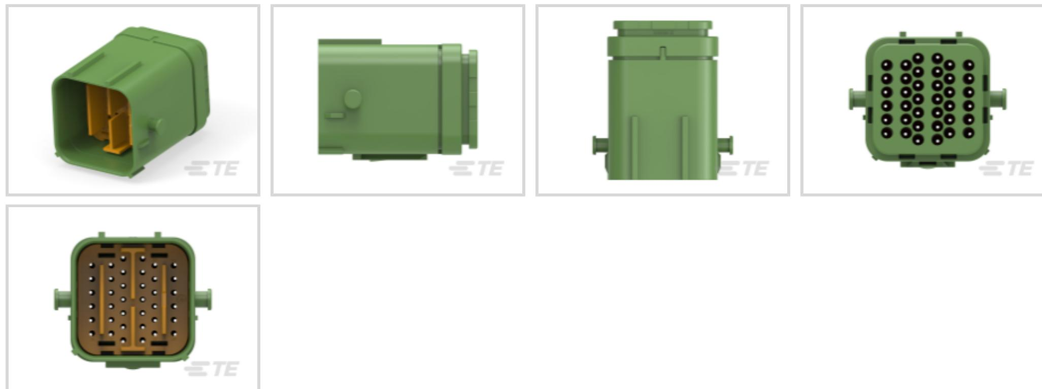
Connector System: **Cable-to-Cable**Number of Positions: **38**Connector & Housing Type: **Receptacle**Sealable: **Yes**Number of Rows: **6**
