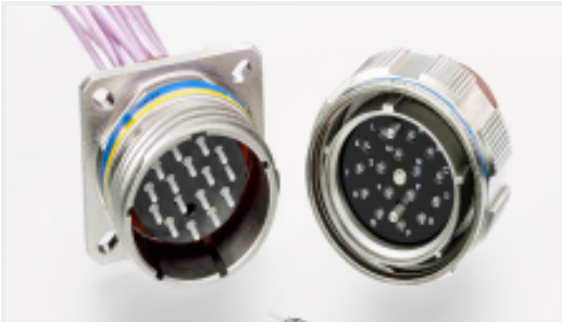
TE Part #YMC8010-Z-21-16PN0 ARINC 801, TYPE 1 RECEPTACLE CONNECTOR
