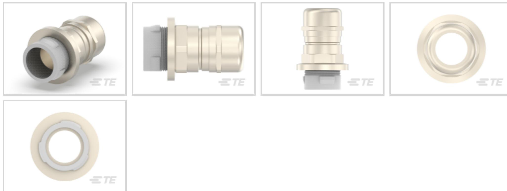
Cable Gland Product Type: **Cable Gland**Cable Gland & Accessory Style: **Snap-In**Primary Product Material: **Brass**Clamping Diameter Range: **11 – 15 mm**Primary Product Plating Material: **Nickel**[All Snap-In type Metal Cable Glands \(15\)](#)
